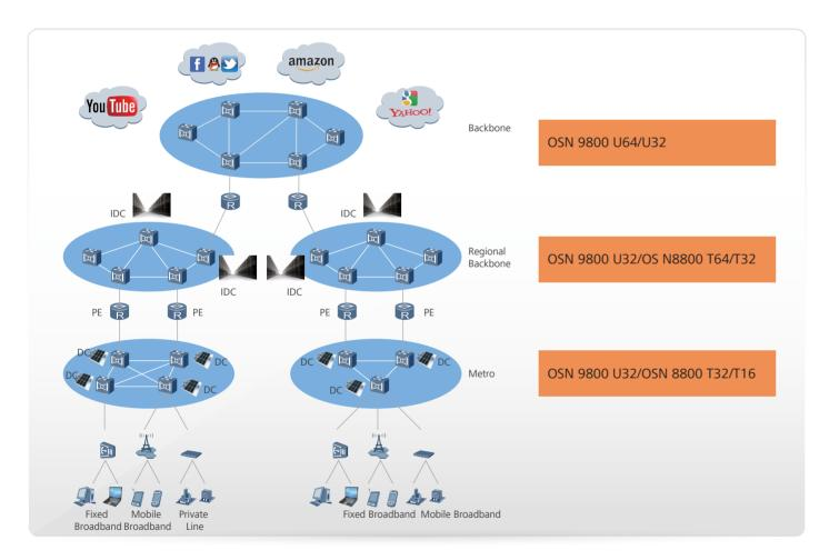
The OptiX OSN 9800 product series is Huawei's next-generation OTN platform for converged packet-optical, intelligent, and optimized networks. These high-performance switching engines offer up to 12.8T cross-connection capacity and feature a universal switching matrix for easy upgrades to 25.6T in a single chassis.
